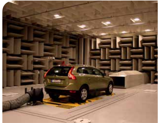
Volvo VSAC showing exhaust and forced air cooling duct (FACD)
