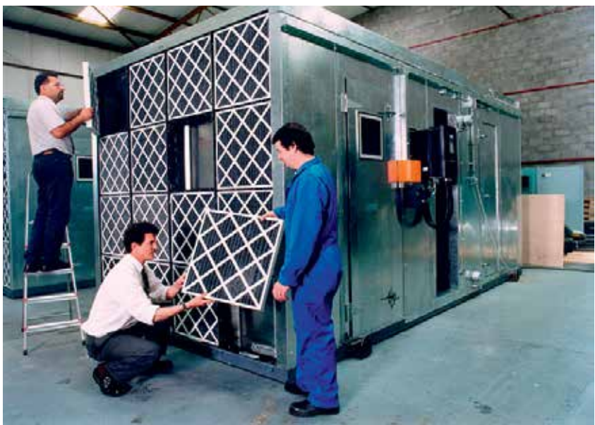
IAC acoustic AHU during assembly
