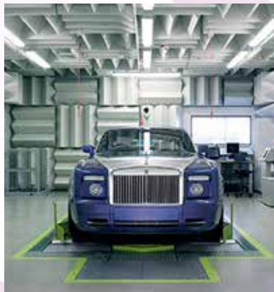
Bespoke shake & rattle facility featuring IAC Metadyne® anechoic wedges at Rolls Royce, UK
