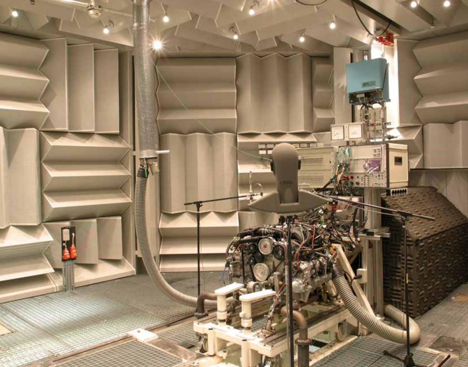
Engine noise test cell, Porsche, Germany
