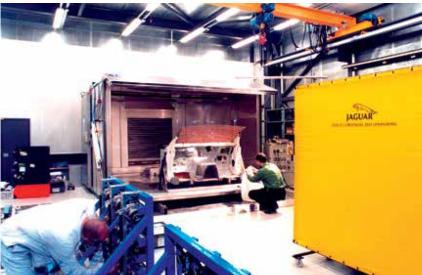
Airbag in-vehicle testing chamber, Jaguar, UK
