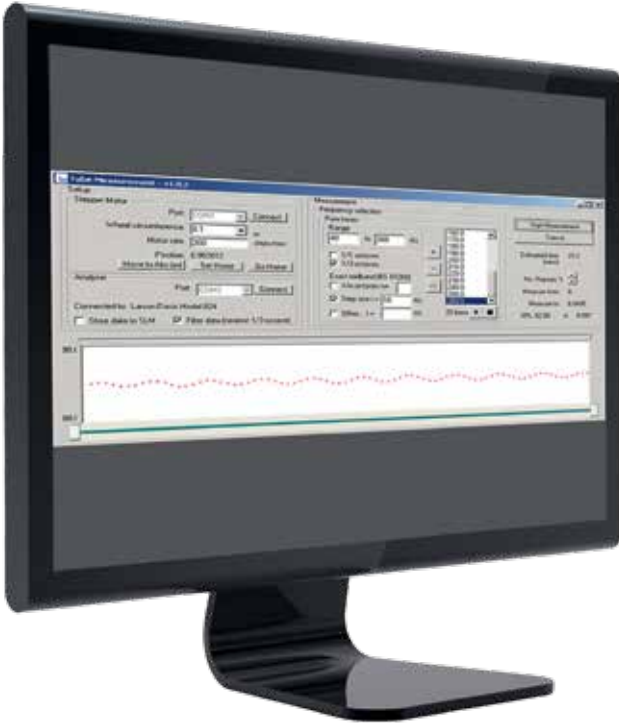
Typical view of IAC's data acquisition system for impedance tube testing
